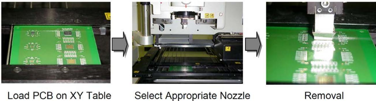
**Figure 3—Removal of Defective Component**
