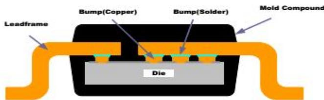
**Figure 2: Flip Chip on Leadframe Structure**
