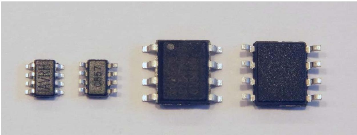
**Figure 1: SOT23 and SOIC Packages**
