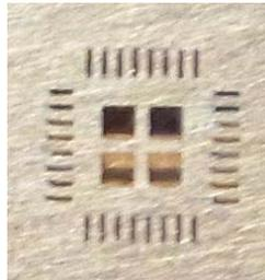
Figure 12: QFN Solder Stencil
