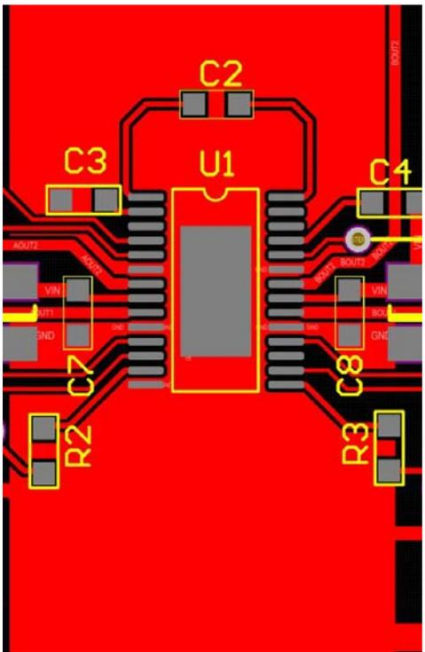
Figure 16: Single-Layer TSSOP Layout
