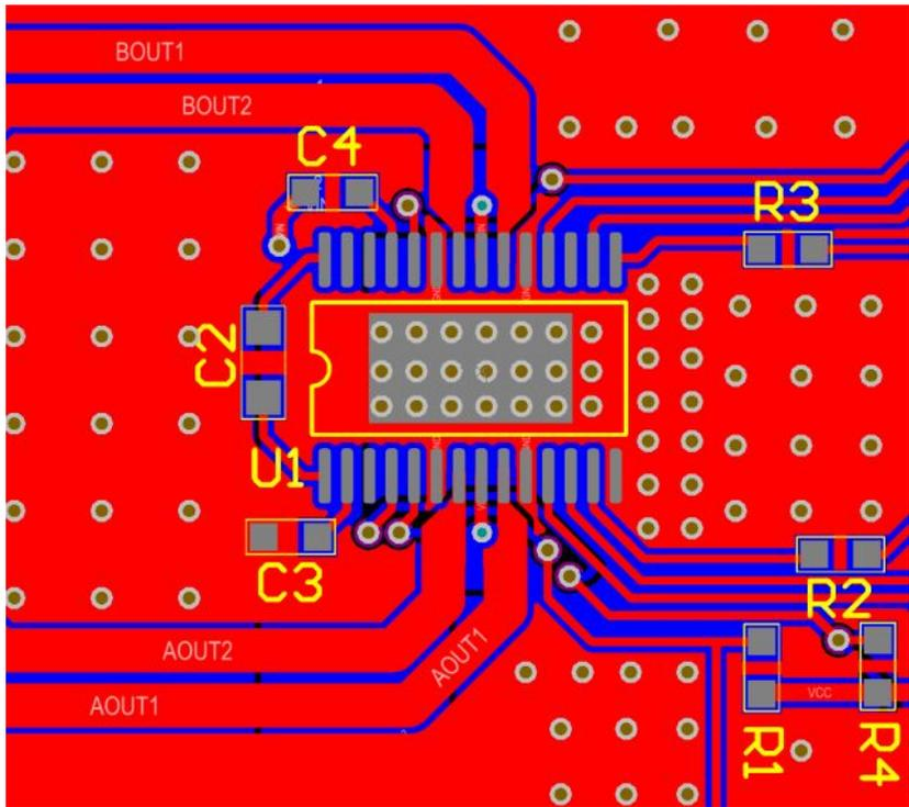
Figure 15: TSSOP PCB Layout
