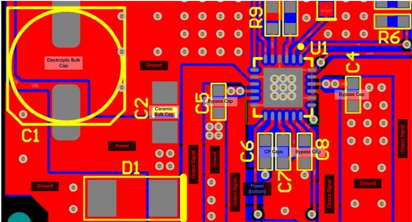
Figure 13: MP6600 Component Placement
