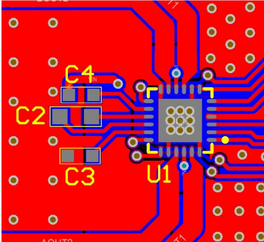
Figure 17: 4mmx4mm QFN Layout
