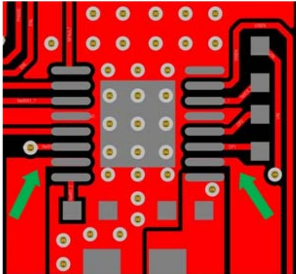
Figure 9: PCB Trace Widening
