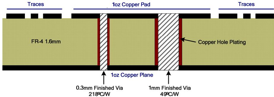
**Figure 10: Via Cross-Section**
