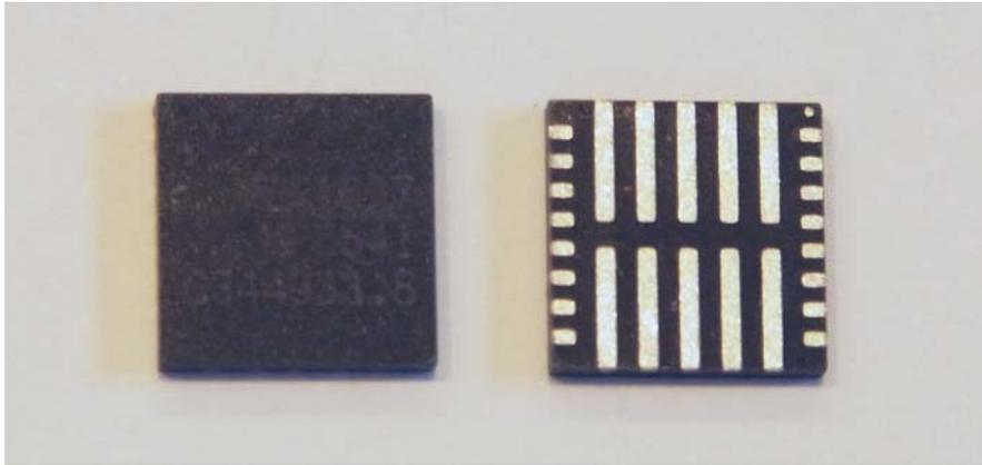
**Figure 5: Flip-Chip QFN Package**
