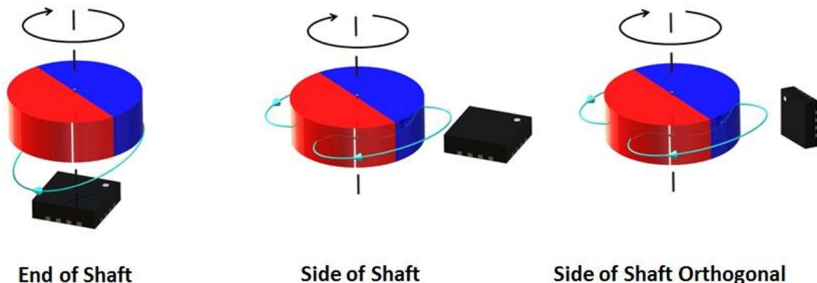
**Figure 5: MAQ430/470 Magnetic Angle Sensor Magnet-Sensing Topologies**
