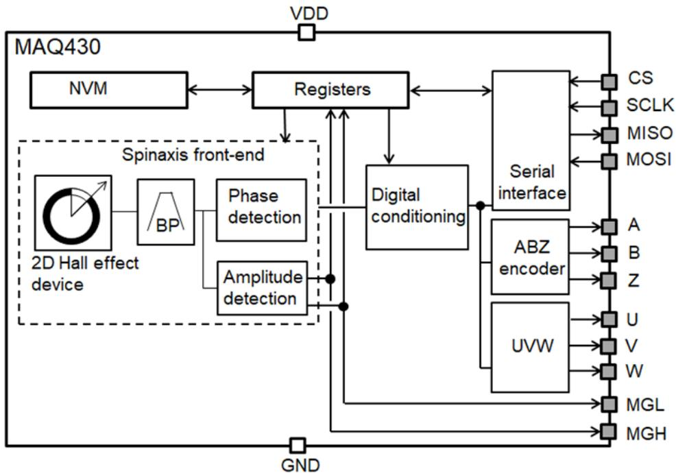
**Figure 4: MAQ430 Magnetic Angle Sensor Block Diagram**
