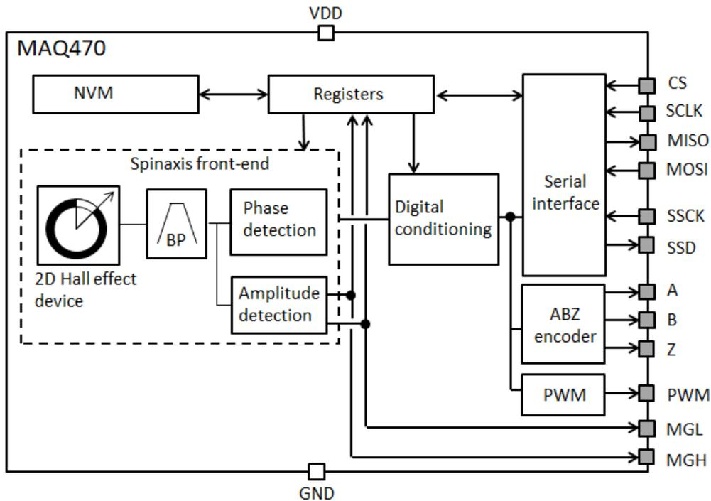
**Figure 1: MAQ470 Magnetic Angle Sensor Block Diagram**
