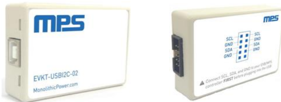
Figure 3: EVKT-USBI2C-02 Communication Interface
