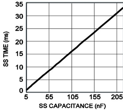
**Figure 2: Recommend SS time vs SS Capacitance**
