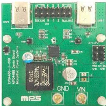
(L x W x H) 5cm x 5cm x 1.7cm (Four Layer PCB/2oz per layer)
