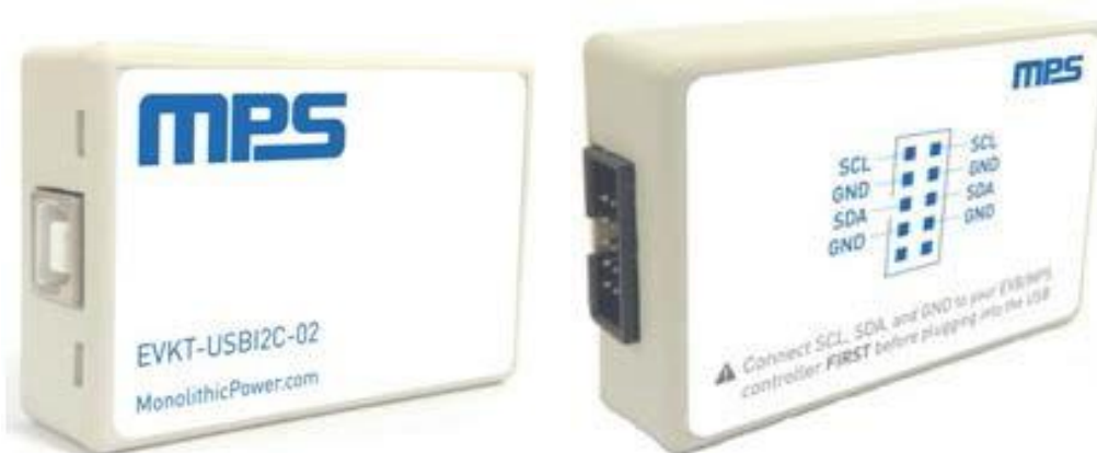
Figure 3: EVKT-USBI2C-02 Communication Interface
