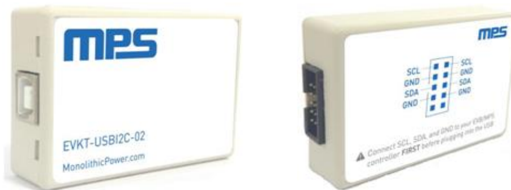
Figure 3: EVKT-USBI2C-02 Communication Interface
