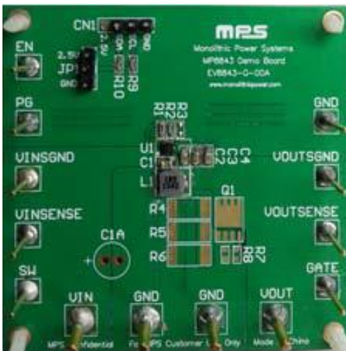
Figure 2: EV8843-G-00A Evaluation Board
