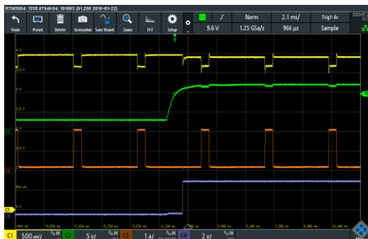
Figure 31: Battery Transition V_{IN} = 0V to 12V , I_{OUT} = 80mA to 2A
