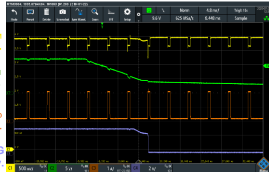
Figure 30: Battery Transition V_{IN} = 12V to 0V , I_{OUT} = 80mA to 2A
