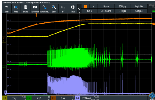
Figure 14: Start-Up through VIN (Buck)
