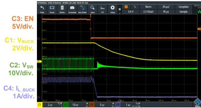
Figure 22: Shutdown through EN (Buck)
