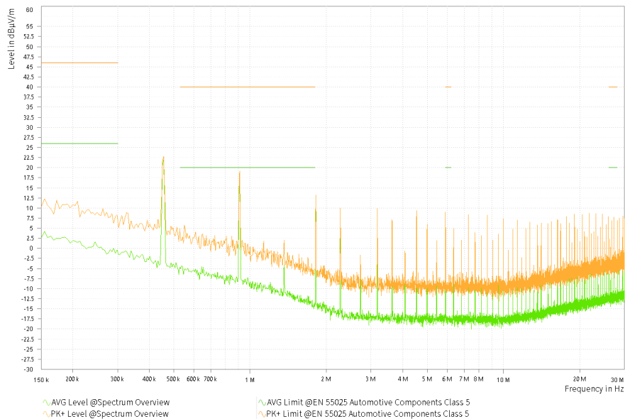
Figure 34: CISPR25 Class 5 Radiated Emissions 150kHz to 30MHz
