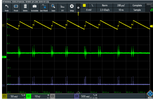
Figure 12: Steady State (Buck)
