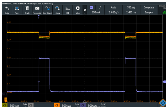
Figure 29: Load Transient (Battery) I_{LOAD} = 80mA to 2A
