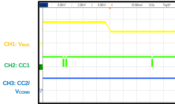
PDO Transition 9V PDO to 5V PDO
