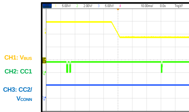
PDO Transition 15V PDO to 9V PDO
