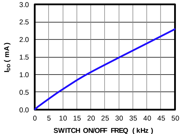
I_{DD} Vs. Switch On/Off Frequency
