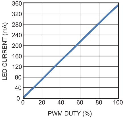
PWM Dimming Curve
