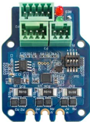
Motor Control PCBA
