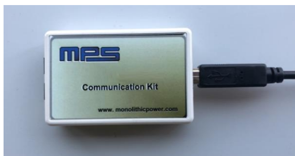
Figure 19: USB to UART Communication Interface (FT485R-KIT)
