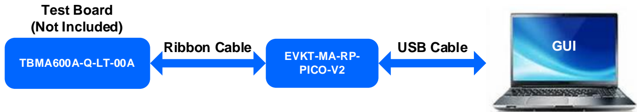
Figure 1: EVKT-MagAlpha-MagDiff Evaluation Kit Set-Up
