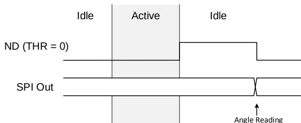
Figure 37: Using the ND Pin as a Flag for Data Updates (THR = 0)
