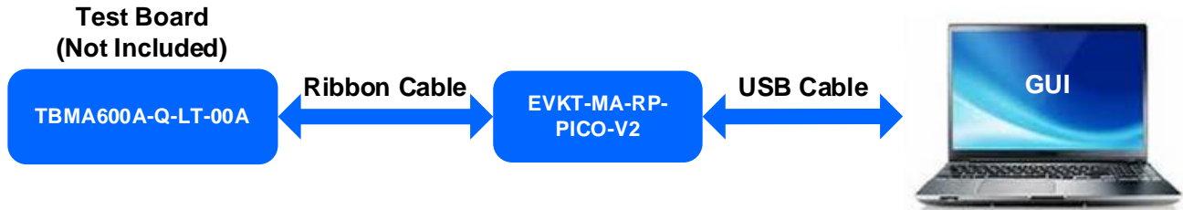
Figure 1: EVKT-MagAlpha-MagDiff Evaluation Kit Set-Up
