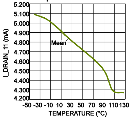
I_DRAIN_11 vs. Temperature Chart
