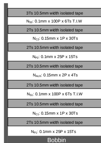
Figure 12: Winding Diagram
