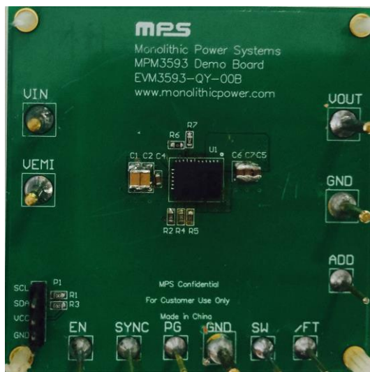
Figure2: EVM3593-QY-00B Evaluation Board
