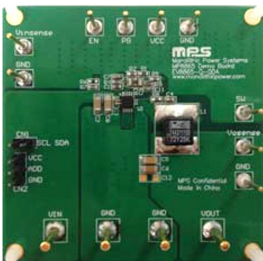
Figure 2: EV8865-Q-00A Evaluation Board
