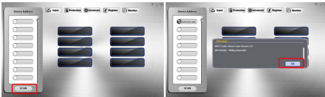
Figure 2: MP5920 Scan Operation
