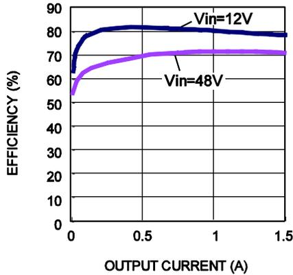
**Efficiency @  $V_{OUT} = 5V$**
