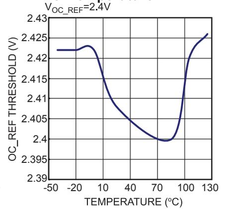
**LSS Current Limit Threshold vs. Temperature**
