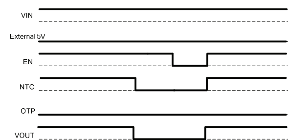
Figure 3: Normal Mode without external 5V \rightarrow NTC protection Mode \rightarrow EN Restart
