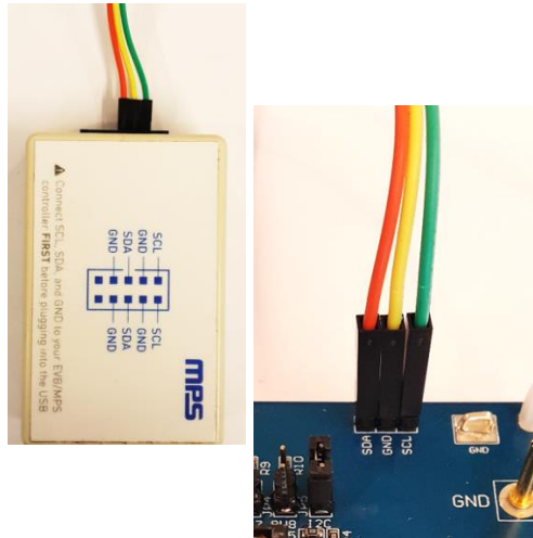
Figure 6: EVB to MPS I 2 C Communication Interface Wire Connection
