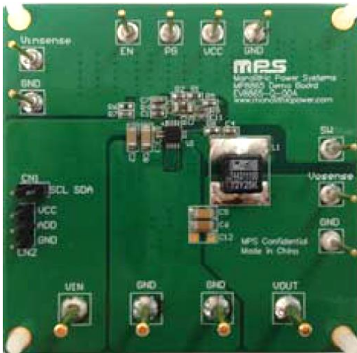
Figure 2: EV8865-Q-00A Evaluation Board
