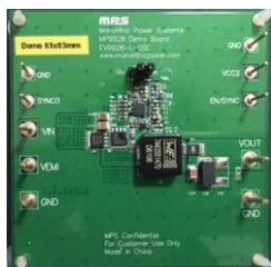
(L x W x H) 8.36cm x 8.36cm x 0.8cm (Four Layers)
