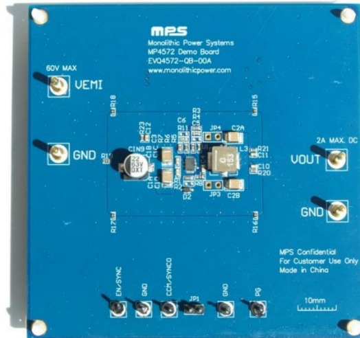
Figure 2: EVQ4572-QB-00A 4-Layer Evaluation Board (8.9cmx8.9cm)
