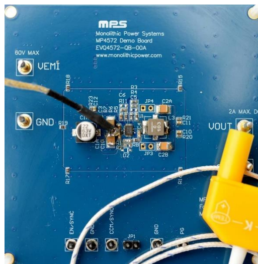
Figure 3: Soldering a Thermocouple to the PCB
