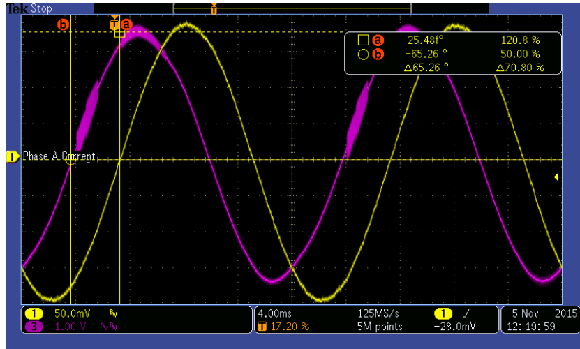
Figure 8: Voltage and Current at No Load
