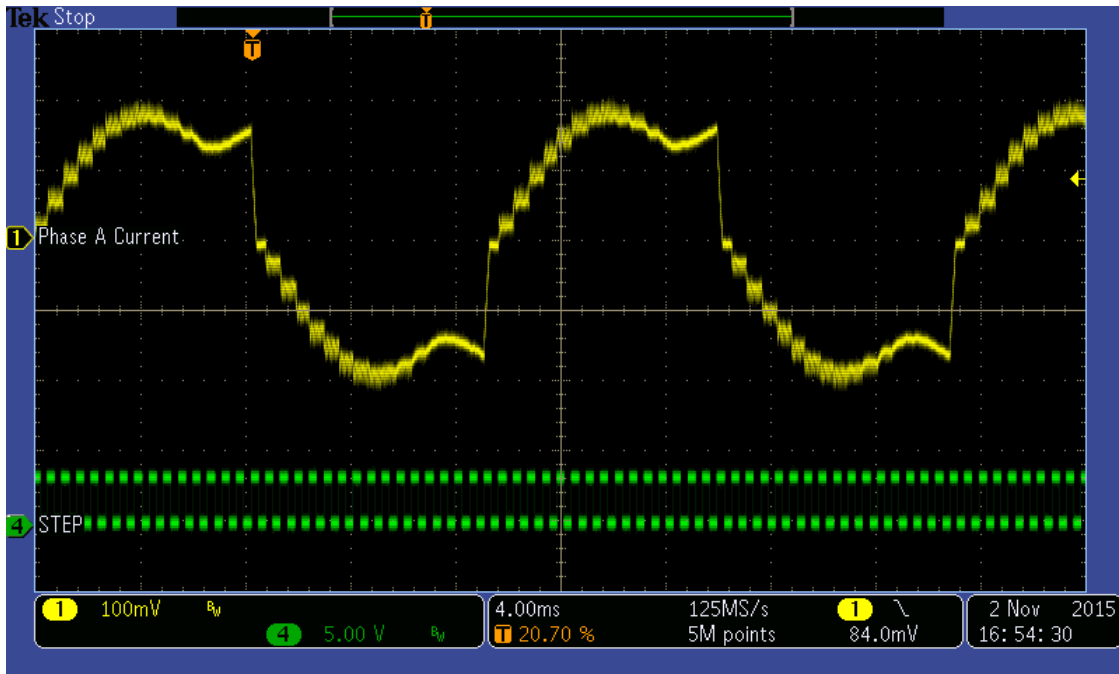
Figure 3: Current Distortion in Slow Decay Mode
