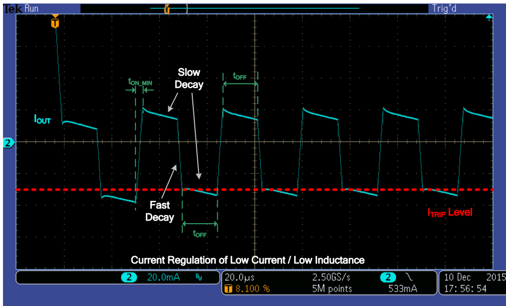
Figure 7: MP6500 Auto-Decode at Low Current
