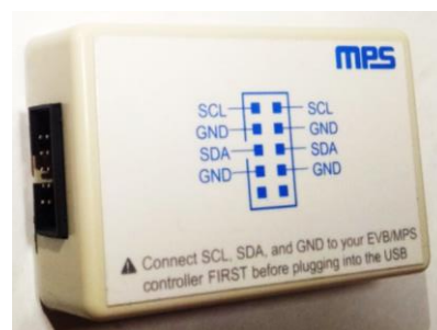
Figure 3: EVKT-USBI2C-02 Communication Interface
