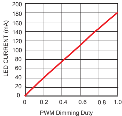
LED Current vs. PWM Dimming Duty
