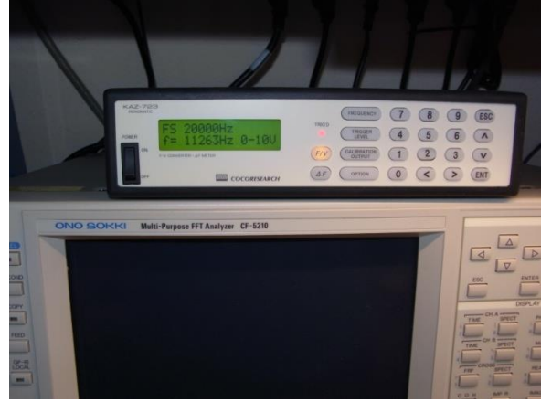
Figure 10: KAZ-723 F/V Converter
